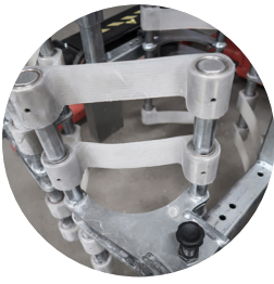
Specially developed polyurethane gripping pads
